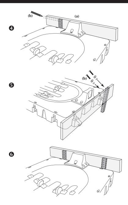
Note: If mounting port to wooden floating dock use 3/8" (9 mm) Lag Bolts (screw based)
