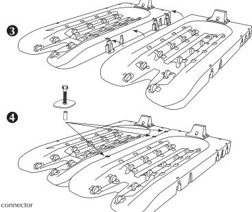
Note: Check all bolts every three months or as needed to insure all connector hardware is securely fastened.
