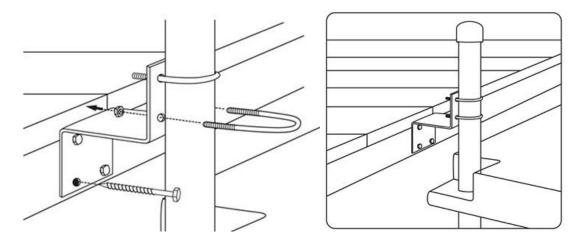
Recommended hardware: four 1/2 lag screws and four 1/2 washers that are Hot Dipped Galvanized
